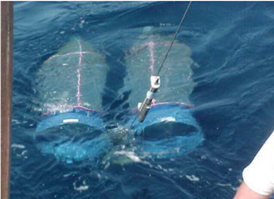
Figure 1. Bongo nets used to sample larval fish in plume and on shelf; Microcat CTD on wire records T, Salinity and depth of tows.
