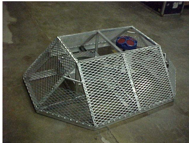
Figure 1: NCSU trawler proof ADCP cage
